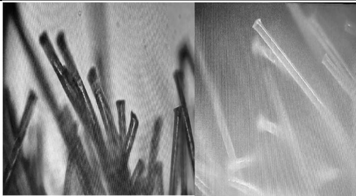
Figure 1 and 2 Nylon hollow fibres at the broken end of test swabs
